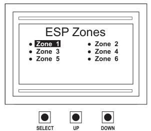
The factory default for all zones is active ESP function as indicated by the bullet (•) next to each zone. To deselect a zone, press the UP or DOWN button until the bullet disappears.
