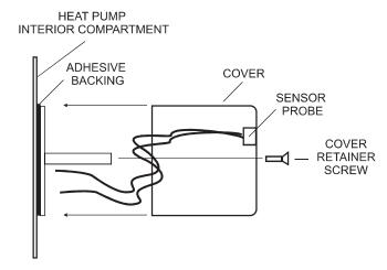
Mount the sensor inside the heat pump cabinet to avoid direct sunlight, freezing rain or snow. The sensor requires separate 18-2 thermostat wire. Connect the sensor leads using wire nuts. Land the other end to the SENSOR screw terminals marked OT on the panel.
