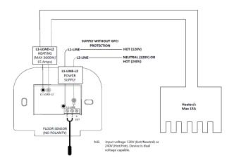
WIRING DIAGRAM 208V & 240V
