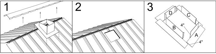
Remove ridge cap. Place ridge flashing over existing metal roof and trace using the inside of the duct as template.
