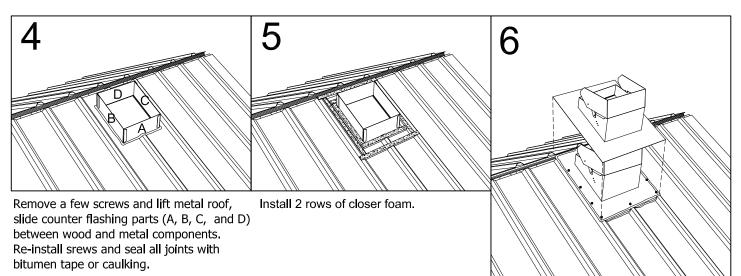
Replace ridge cap over flashing. Place ventilator head over the slope flashing, making sure it is level and fasten with screws provided into each of the perforated holes. (Model 301 shown)
