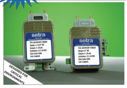
etra Systems Model 269 pressure transducers sense differential pressure and convert this pressure difference to a proportional electrical output for either unidirectional or bidirectional pressure ranges. The 269 Series is offered with a 4 to 20 mA analog output.
