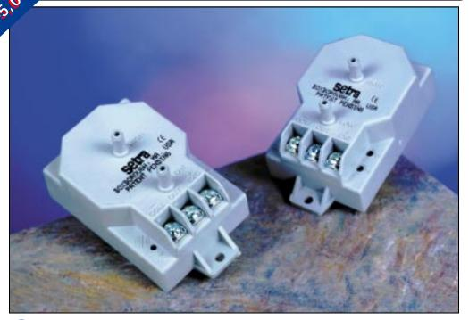
etra Systems 265 pressure transducers sense differential or gauge (static) pressures and convert this pressure difference to a proportional electrical output. The 265 is offered with a high level 0-5 VDC output or a 4-20 mA output. It is also offered with 0-5 or 0-10 VDC output in the 24 VAC excitation version.
