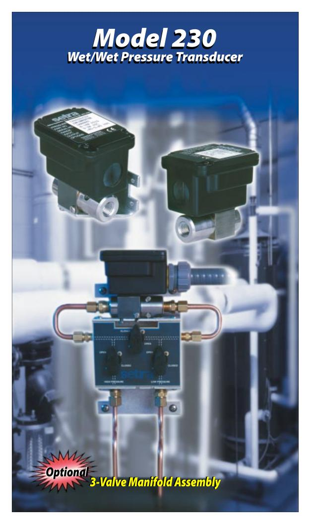
etra Systems Model 230 is a high output, low differential pressure transducer designed for wet to wet differential pressure measurements of liquids or gases. A fast-response capacitance sensor and signal conditioned electronic circuitry provide a highly accurate, linear analog output proportional to pressure. Both unidirectional and bidirectional pressure ranges are available for applications with line pressure up to 250 psig.
