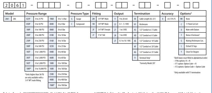
Ordering Example: 2061025PG2M11048CN - Model 206, 0 to 25 PSIG, Gauge pressure, 1/4" NPT Male fitting, 4 to 20 mA output, 4' Cable Length, ±0.13% FS Accuracy, 11 Point Cal Cert option
