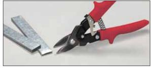
The Max2000 Bulldog Snip features shorter blades with a serrated lower jaw for controlled notching and trimming out to the blade tip in layered sheet metals and metal seams.
