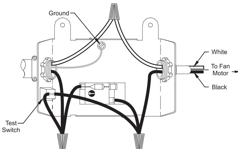
9. **WARNING!** Turn off power before connecting power wires to ventilator. Your power feed wire should be 14 gauge or larger wire size (two wires plus ground). Take from thermostat box and bring to power distribution panel. Feed through bushing and connect to 15-amp circuit breaker.
