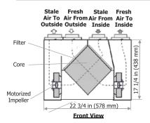
Note: Front clearance of 25 in (635 mm) is recommended for servicing unit. All ducts use 5 in (125 mm) oval collars, balancing dampers are located on all collars.
