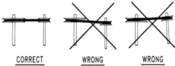
FIGURE 1 PULLEY ALIGNMENT
