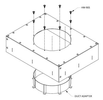
Installing the Duct Adapter:
