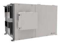
The SHR 450 Commercial Heat Recovery Ventilation system (HRV) complements today's tight buildings. Fantech Heat Recovery Ventilators (HRV) are designed to supply air into a building while exhausting an equal amount of contaminated air to the outside. The aluminum heat exchanger core transfers sensible energy between air streams resulting in tempering of the supply air and reduced loads on the HVAC system.
