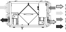
fresh air to inside fresh air from outside stale air from inside stale air to outside
