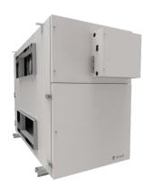
The SHR 1400 Commercial Heat Recovery Ventilation system (HRV) complements today's tight buildings. Fantech Heat Recovery Ventilators (HRV) are designed to supply air into a building while exhausting an equal amount of contaminated air to the outside. The aluminum heat exchanger core transfers sensible energy between air streams resulting in tempering of the supply air and reduced loads on the HVAC system.
