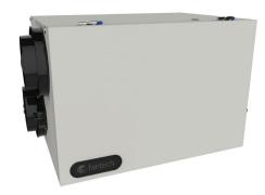
Fantech's, SER 200 is an Energy Recovery Ventilator designed for higher static pressure applications. The unit brings a continuous supply of fresh air into a home while exhausting an equal amount of contaminated air. The energy recovery core at the center of the unit transfers heat and moisture from incoming air to the outgoing air that was cooled and dried by the building's air conditioner.
