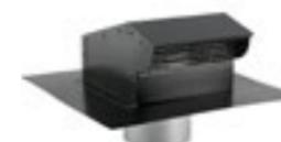
**Roof Cap RC** for installation on sloped roofs are assembled with pre-painted black painted steel sheet. They include 1/4" discharge screen, aluminum backdraft damper with rubber gasket, and 3" duct collar extension.
