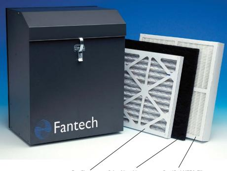
**Pre-filter** Captures larger particles. Odor Absorbing Carbon Filter captures and neutralizes odors from cooking and tobacco smoke. **Certified HEPA Filter** High Efficiency Particle Filter tested and certified to be 99.97% effective down to 0.3 microns. Filter has a long life cycle. Replace once every two years.
