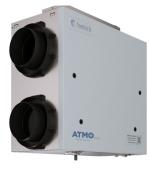
Powered by EC motors, the ENERGY STAR<sup>®</sup> and HVI certified ATMO™ 300E-EC fresh air appliance with energy recovery (ERV) uses a water vapor transport, durable, polymer membrane that transfers heat and moisture to the incoming air. This process helps to temper the incoming air and to maintain comfortable humidity levels.
