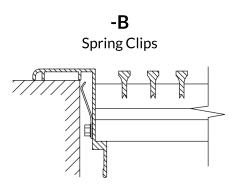
Hidden clips behind the flange to keep the grille secure in the opening. Only suitable for floor & sill applications.
