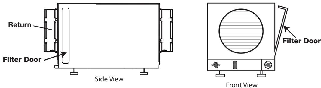
Step 2: Remove the filter by gently pulling straight out of the unit. Insert new filter by gently pushing it straight into the unit. Make sure the AIR FLOW arrow on the filter is pointing into the unit.
