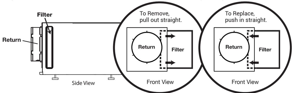
Step 3: Replace filter door ensuring the opening is fully covered.
