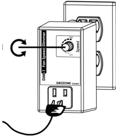
In LOW position, this controller will NEVER turn your unit OFF and will keep your unit running at Idle speed (also called minimum speed).
