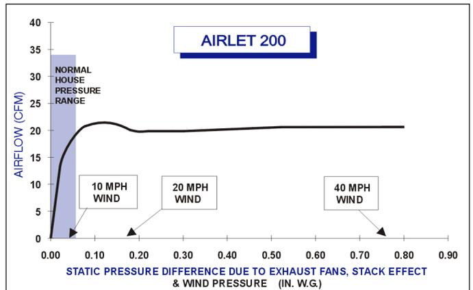
AIRLET™ 200 make-up air inlets are self-regulating. The controlling element is a plastic damper that automatically adjusts the free opening to provide a draft-free regulated amount of incoming air, independent of wind pressure. (See performance charts at right.)
