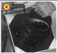
Pull band around perimeter of unit, unneeded sections will break off to be recycled or discarded
