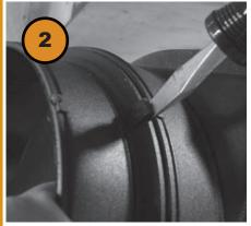
Place flat screwdriver head into the appropriote slot to remove unneeded collar(s).
