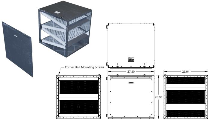
Units are in inches, The Pressure Drop over the MERV13 Filters is 0.2" W.C. @ 4000CFM.
