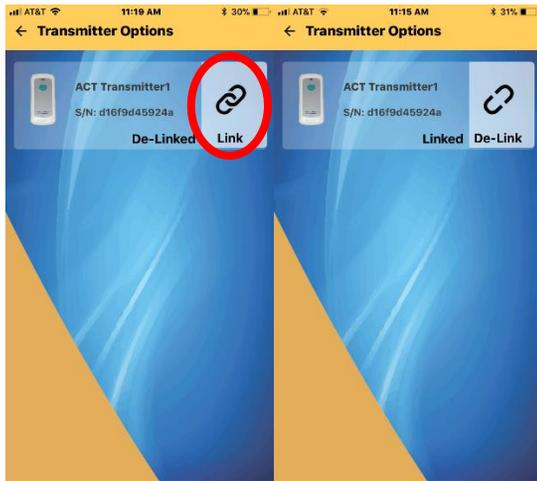
10. From the main menu you can check the status of all of your devices. To verify the pairing, tap the "Receiver/Hub" button, then tap the "Transmitter Options" button. This will show you the Transmitters linked to your Receiver. Make sure all of the Transmitter(s) are shown on this screen and that they all are "Linked" as shown below.
