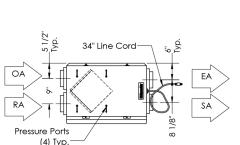
22 1/4" Minimum Service Area (Door can be Removed from Hinges.) 23 7/8" Case 18 1/2" Minimum Service Area Overall Door Swing 20" Control Terminal
