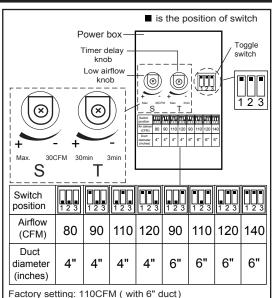
Factory setting: 110CFM ( with 6" duct)
