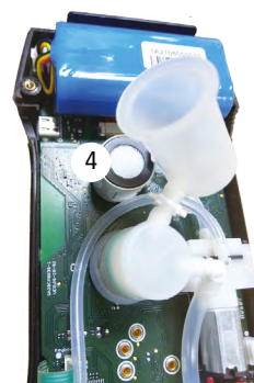
New sensor connected to electronic board
