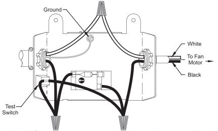
WARNING! Turn off power before connecting power wires to ventilator. Your power feed wire should be 14 gauge or larger wire size (two wires plus ground). Take from thermostat box and bring to power distribution panel. Feed through bushing and connect to 15-amp circuit breaker.
