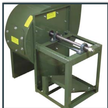
MOTOR AND DRIVE COMPARTMENT WITH COVER REMOVED TO ILLUSTRATE 3 SIDE MOTOR ACCESS AND SLOPED MOTOR BASE FOR BELT TENSIONING.
