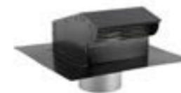
**Roof Cap RC** for installation on sloped roofs are assembled with pre-painted black painted steel sheet. They include 1/4" discharge screen, aluminum backdraft damper with rubber gasket, and 3" duct collar extension.
