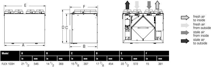
Dimensional information is in inches. Clearance of 14" (356mm) in front of the unit is recommended for removal of core. All units feature three foot plug-in power cord with 3-prong plug.
