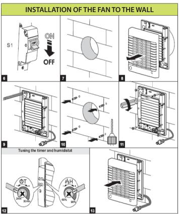
Cord set not included in all models. **Figure 10** shows the adjustment of the timer and dehumidistat (not available on model TTW-100).
