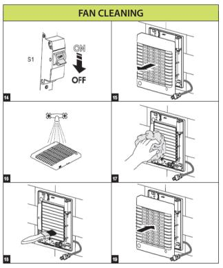
Fan surfaces need to be cleaned regularly from dirt and dust. **See Figures 14-19**. Clean with a soft cloth, using a solution of water and a cleaning agent. Avoid getting liquid on electric motor. After cleaning, the surface must be wiped dry.
