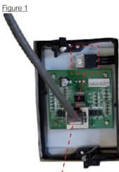
The indoor temperature sensor is located inside of TSP wall switch
